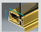
Series 407 has been designed to go into sub-head, sub-sill and sub-jambs. Sub-sill shown above.
